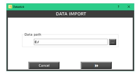
Select the folder where your data is saved. If Datastick software found a USB drive connected to your computer, it will select automatically.
